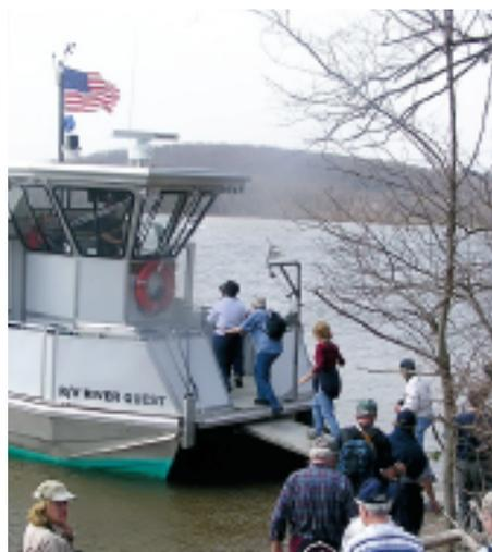
**A ramp under the bow can be pulled out when the boat is beached, allowing passengers to easily board and depart the boat.**
